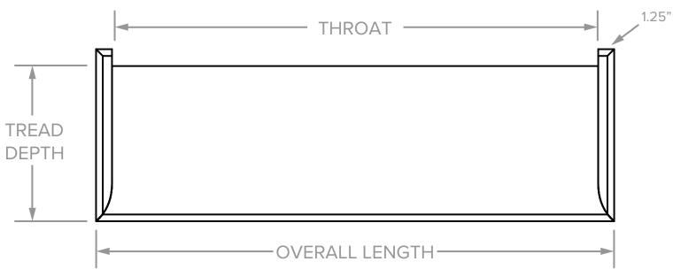
\*OVERALL LENGTH SHOULD BE 2.5" LONGER THAN THE THROAT TO ACCOUNT FOR RETURN END THICKNESS
